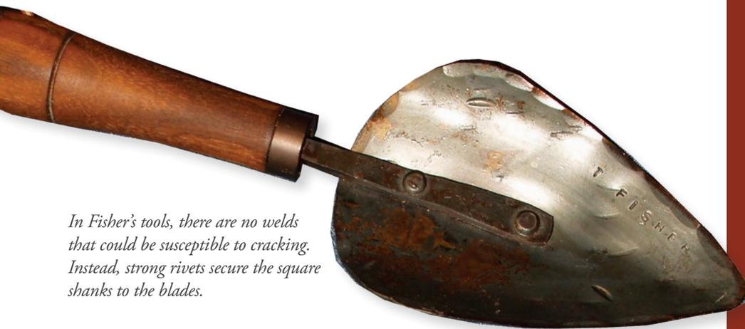
*In Fisher's tools, there are no welds that could be susceptible to cracking. Instead, strong rivets secure the square shanks to the blades.*
