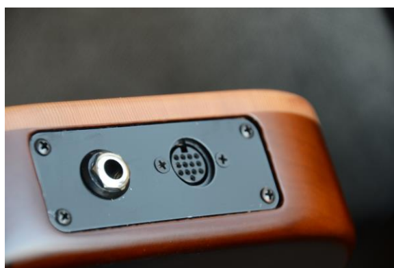
LEFT: A Roland GK-3 in custom middle position. RIGHT: A Godin acoustic guitar with common 1/4" and multichannel 13pin output.
