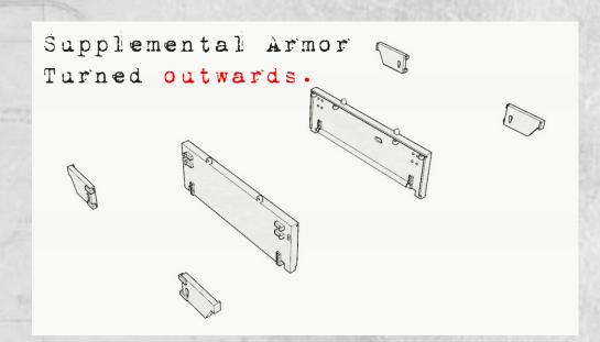
We recommend you sand the connecting point before gluing the parts in place. This will make for a stronger bond.
