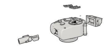
We recommend you sand the connecting points before gluing the parts in place. This will make for a stronger bond.
