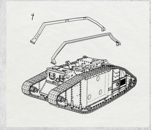
We recommend you sand the connecting points before gluing the parts in place. This will make for a stronger bond.
