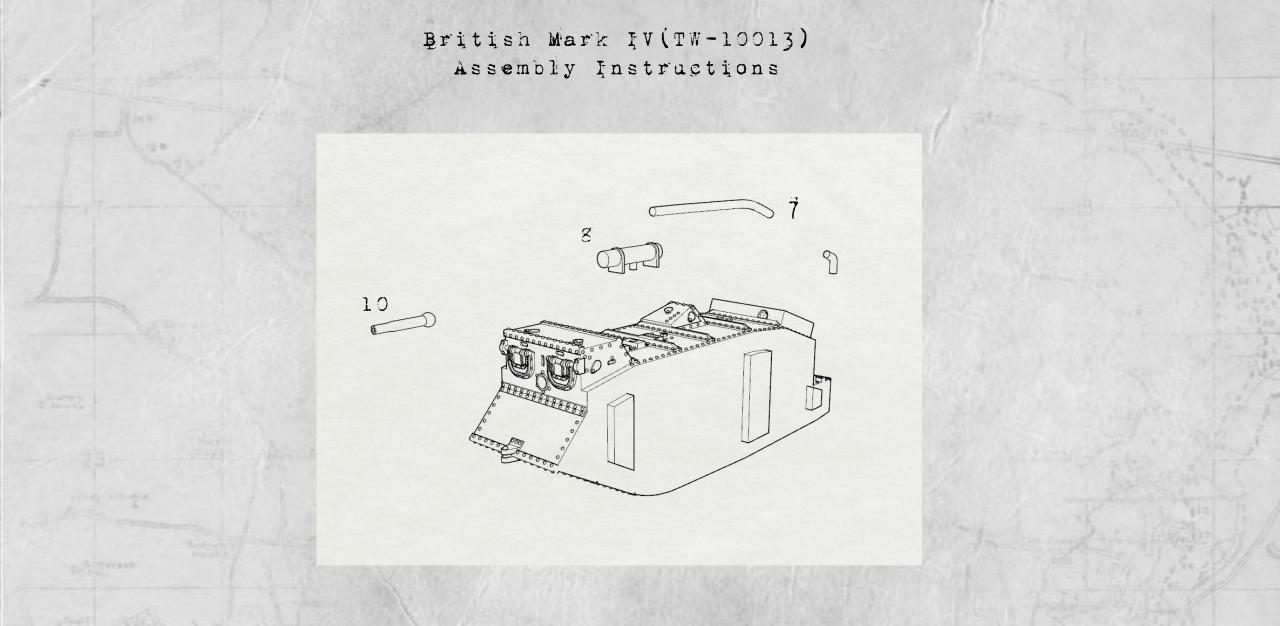
We recommend you sand the connecting points before gluing the parts in place. This will make for a stronger bond.
