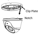
Figure 2-6 Disassemble the Camera
