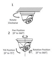
Figure 2-15 3-axis Adjustment
