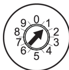
Figure 3.1: Address switch set to 1
