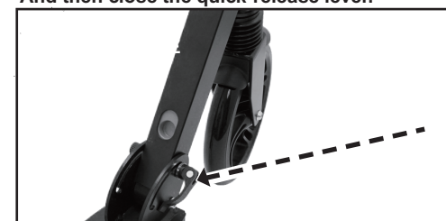
Open the quick-release lever.
