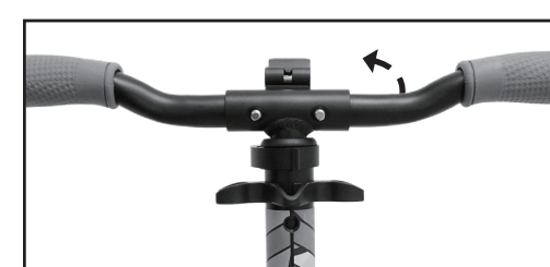
Open the handle bar clamp.
