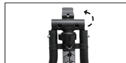
Open the handle bar clamp.
