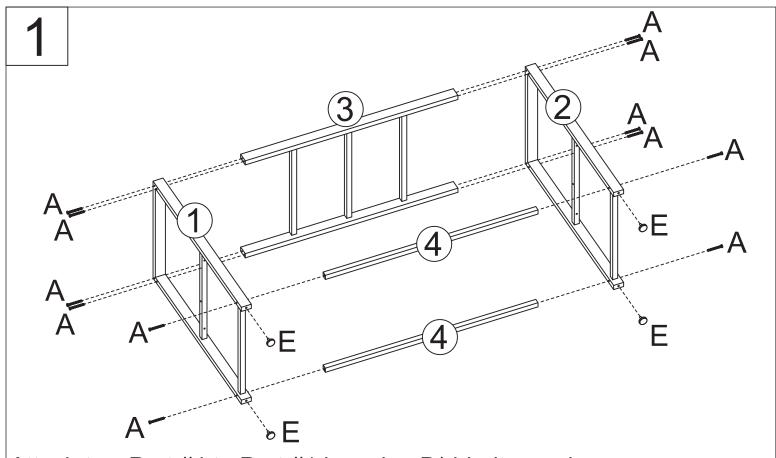
Attach two Part #4 to Part #1 by using D\*4 bolts as shown **Attention: three circled parts face the same side when assembly**
