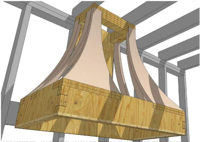
\*IF NEEDED, USE STEEL HANGER STRAP TO SECURE RANGE HOOD
