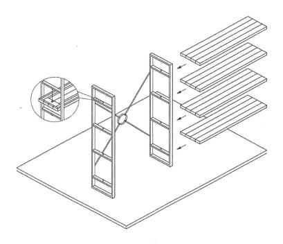
STEP 3 Fit the individual shelf into the location points on the Metal frame
