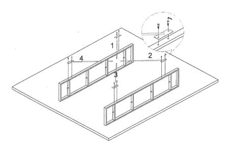
STEP 1 Insert metal (1, 2, 3, 4) into Metal frame by using Bolt (A) & Washer (B).
