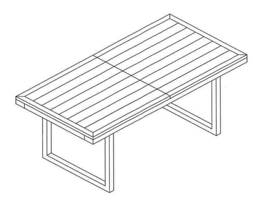
STEP 4 Carefully turn the table over on to its feet, and fully tighten all bolts.
