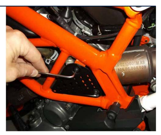
Use allen key (hex key) #5 to remove the clamp bolts
