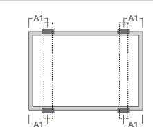
Use four clamps on the long side. Mounting rails run perpendicularly to the long side frame.
