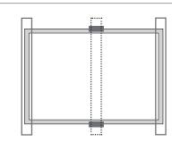
Use two insertion profiles running perpendicularly to the long side frame. An additional support bar should be placed below the module. Use two clamps on the support bar.
