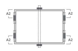
Use four clamps on the short side and two clamps on the long side. An additional support bar should be placed below the center of the module.
