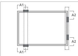
Use two clamps on the long side and two clamps on the short side.
