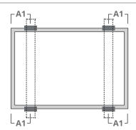
Use four clamps on the long side. Mounting rails run perpendicularly to the long side frame.
