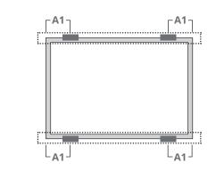
Use four clamps on the long side. Mounting rails run parallel to the long side frame.
