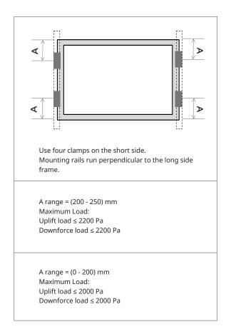
Rail-less clamping for CS3K-P, CS3K-MS, CS6K-P, CS6K-M, CS6K-MS, CS1K-MS, CS1H-MS
