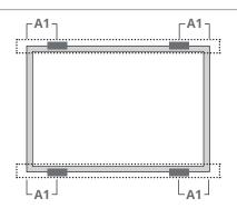
Use four clamps on the long side. Mounting rails run parallel to the long side frame.
