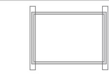
Use two insertion profiles running perpendicularly to the long side frame.
