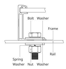
Modules should be bolted at the following hole locations depending on the configuration and loads:
