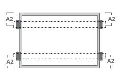
Use four clamps on the short side. Mounting rails run parallel to the long side frame.
