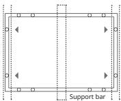
Maximum Load: Uplift load ≤ 2400 Pa Downforce load ≤ 5400 Pa
