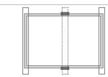
Use two insertion profiles running perpendicularly to the long side frame. An additional support bar should be placed below the module. Use two clamps on the support bar.
