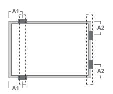
Use two clamps on the long side and two clamps on the short side. Mounting rails run perpendicular to the long side frame.
