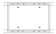
Maximum Load: Uplift load ≤ 2400 Pa Downforce load ≤5400 Pa
