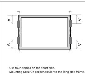
A range = (200 - 250 mm) Maximum Load: Uplift load ≤ 1400 Pa Downforce load ≤ 1400 Pa
