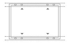
Maximum Load: Uplift load ≤ 2400 Pa Downforce load ≤4000 Pa
