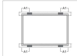
Use four clamps on the long side. Mounting rails run parallel to the long side frame.
