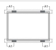
Use four clamps on the long side. Mounting rails run parallel to the long side frame.
