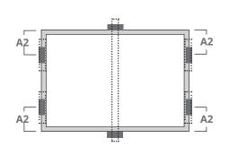
Use four clamps on the short side and two clamps on the long side. An additional support bar should be placed below the center of the module.
