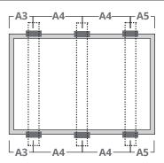
Use six clamps on the long side. Mounting rails run perpendicularly to the long side frame.
