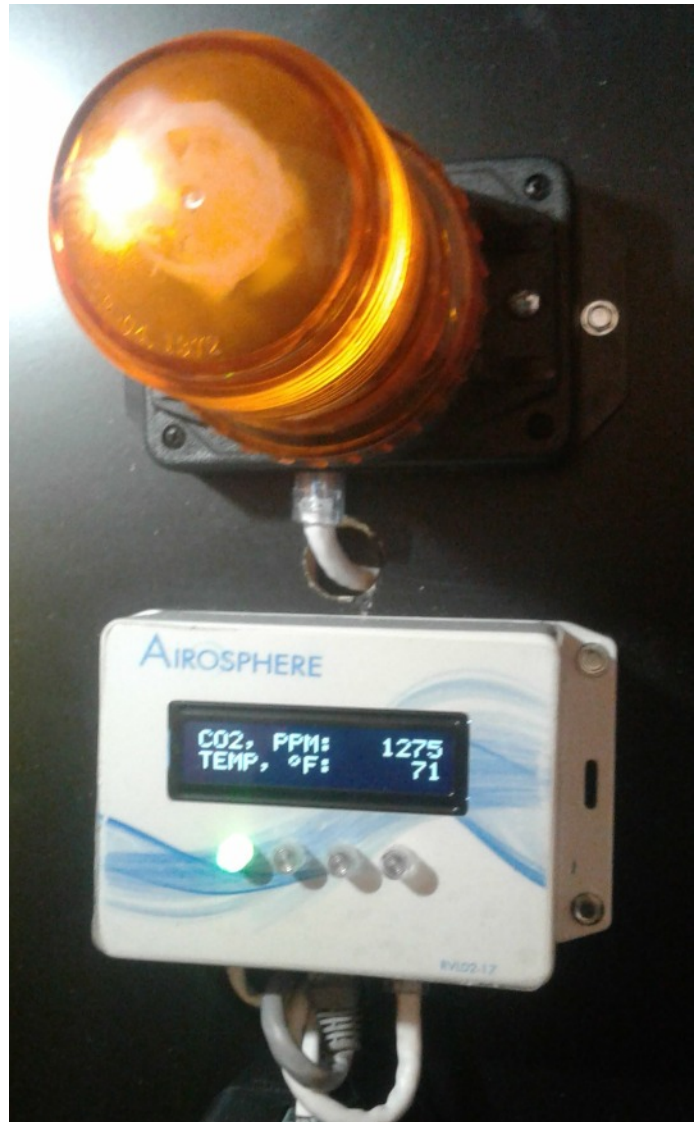
Optional remote sensor or repeater display, with audible alarm and strobe
