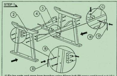
1) Fix leg parts and cross bars together using 60mm bolt (B) screw and barrel nut (C)
