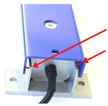
A gap of at least ¼ inch must be maintained between the floating top section and the main structure for the load bars to work correctly
