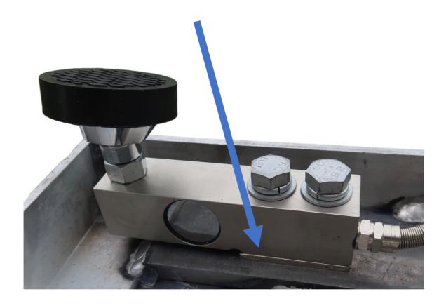
Ensure a good clearance gap is maintained (at least 1/8 of an inch)
