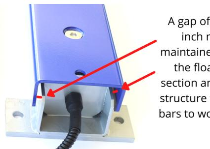
A gap of at least ¼ inch must be maintained between the floating top section and the main structure for the load bars to work correctly
