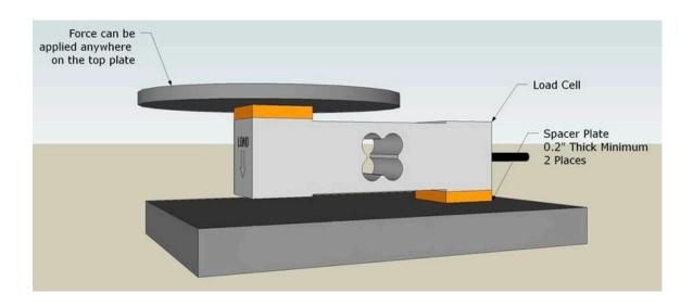
If installing on a timber platform – add a channel so the load cell has more room to take a reading with less chance of touching the platform.
