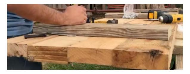
**Step 2**: Turn the platform upside down and use the spacers provided to drill 2 x holes at each corner of the platform. Space these holes and the load cells close to the edge of the platform.
