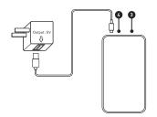
3 Input: Connect the power bank to your USB adapter with the Type-C cable for charging the power bank.
