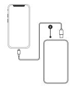
Output: Connect the power bank to your Android device with the Type-C cable for charging your Android device./ Connect the power bank to your iOS device with an MFi cable (not included) for charging your iOS device.
