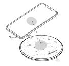
Step 2: Place your mobile device on the top of the product. Ensure it is on the right position/direction.
