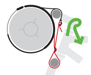
Thread the lower straps under the fork crown, back up and re-thread them through the tri-bar adjusters.
