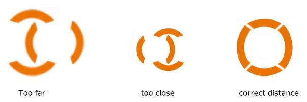
When you are at the correct distance, release the button and keep the thermometer steady for less than one second until the lights flash and the temperature appears on the LCD display. There is no need to concern if the aiming lights are pointed into the eyes: the beams are not laser lights and are absolutely harmless.
