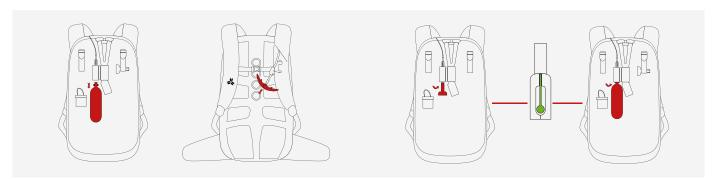
You can practice without actually having to deploy the airbags by simply removing the cylinder from the puncture unit and pulling on the trigger handle. After each practice session, remember to reactivate the trigger system using the reactivation key designed for this purpose.
