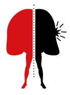
A Reactor backpack is equipped with two airbags separated by an internal divider, creating two independent airbag for increased reliability. Both inflate simultaneously and each has its own independent intake valve.
