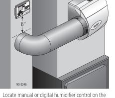
return 6" above the humidifier or bypass duct.
