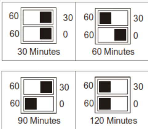
Dipswitch Settings for Selection of Defrost Time
