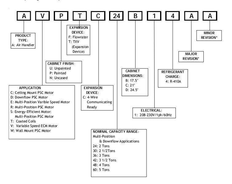
All Airhandlers use DIRECT DRIVE MOTORS. Power supply is AC 208-230v, 60 hz, 1 phase.
