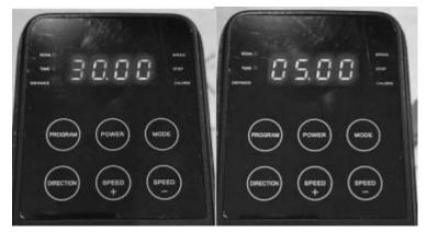
4. After you adjusted working time, you could press button of POWER to start machine. This moment, machine is under manual program and display will show speed 1 at first. You could adjust speed from 1 to 10 via button speed + or speed-. Maximum speed is 10.
