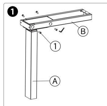
Insert the lifting column into the crossbar, and then use the allen key to insert and tighten the four M6x10 screws.
