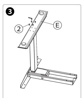
For each leg assembly, attach then screw on the foot base using four M6x16 screws and tighten them using the allen key.
