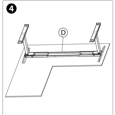
Connect the two crossbars using two central rails. Make sure the frames are properly positioned beneath the desk top.
