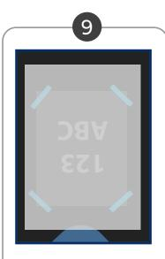
Cover with a sheet of parchment or kraft paper and press at 310°F / 154°C for 30 seconds. Press with med - high pressure.
