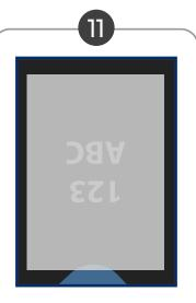
Place garment back on heat press. Cover image with parchment or kraft paper. Press for 10 sec at 310°F / 154°C
