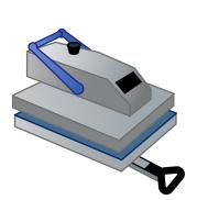
Preheat the closed press to 310°F / 154°C. Wait for the heat press to reach the desired temperature before moving forward.
