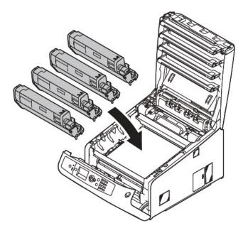
6 Turn the blue lever (7) of the toner cartridge in direction of the arrow fully. Turn the levers of all four 4 toner cartridges.
