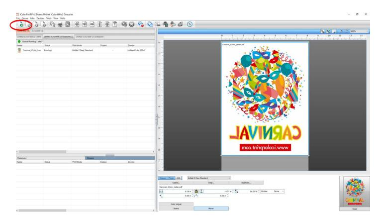
12) There are preloaded images that can used to print a test page. Click **Devices >> Print Test Page** to see the choices. It is suggested that you print a test page upon completion of the setup to confirm the printer has been properly installed. Use [Shift] and [Ctrl] to select multiple pages, and then click OK. More about the uses of each page can be found in the Help Topics file within the ProRIP program as well as the ProRIP User Manual.
