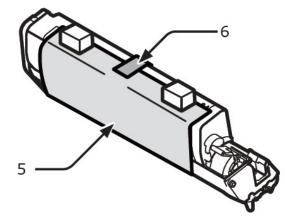
(2) Pull out a protective sheet to the direction of the arrow.
