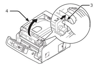
NOTE: The white cartridge that came preinstalled in your machine is already in the locked position. Just remove the protective covering - it is not necessary to turn the blue lever. Doing so can cause toner to spill.
