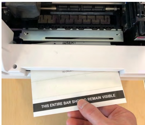
3. Unload label stock from the printer. Insert the cleaning card into the front output of the printer.
