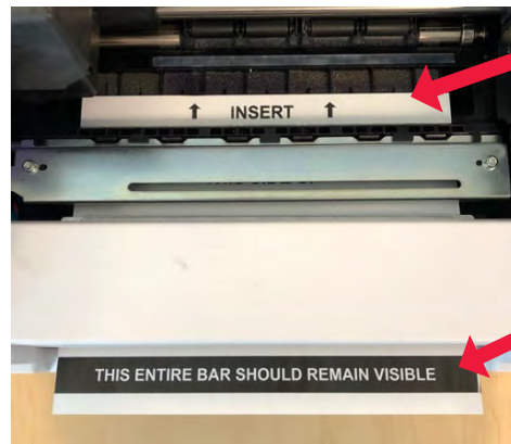
4. When the exposed adhesive strip is aligned with the Output cutter path, open the UNINET IColor PrintHub – select Printer Settings – Advanced. Click on Output Cutter Cleaning. Once the cutter cycles, remove both parts of the card from the printer.
