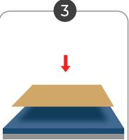
Place a piece of parchment or kraft paper on the bottom plate so you can easily remove the substrate when hot.
