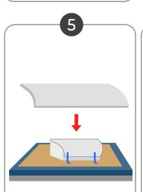
Cover with a silicone pad (.32mm suggested) or the foam pad depending on the substrate in use.
