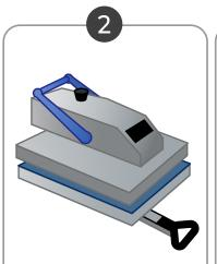
Preheat the closed press to the according temperature (see chart). Wait for the heat press to reach the desired temperature before moving forward.
