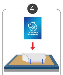
Align the substrate to the printed image & lay flat on press with transfer paper on top. You can apply tape on blank areas of the transfer paper to the lower kraft paper for additional stability.
