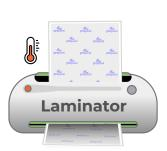
Run the two sheets together through a laminator on med - high heat setting prior to pressing. This will remove any air bubbles. DO NOT use a carrier sleeve.
