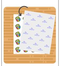
Once the image is printed, place the adhesive sheet on top of the print. The white (adhesive coated) side should be face DOWN.
