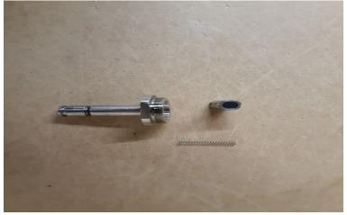
Be sure to clean all parts of the core and valve body with a wire brush and flush thoroughly with water. Once all parts are clean reassemble the core and then hand thread the core back into the valve body and re tighten with an adjustable spanner.
