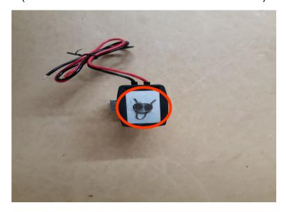
Once you have the clip removed set it aside along with the top plate. Pull the valve body from the coil And set aside 2 of the 3 washers from under it aside with the clip and top plate for reassembly.
