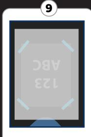
Cover with a sheet of parchment or kraft paper and press at 310°F / 154°C for 30 seconds. Press with med - high pressure.
