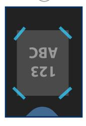
Thread your garment onto the heat press. Align your image on the garment and fix it in place using heat resistant tape.
