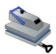
Preheat the closed press to 310°F / 154°C. Wait for the heat press to reach the desired temperature before moving forward.
