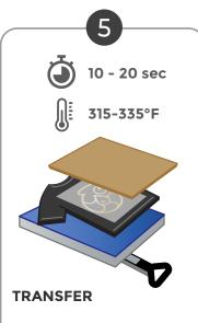
Place the film (print-side DOWN) onto the platen-threaded garment. Cover with silicone pad or parchment paper. Press for 10-20 sec at 315-335°F
