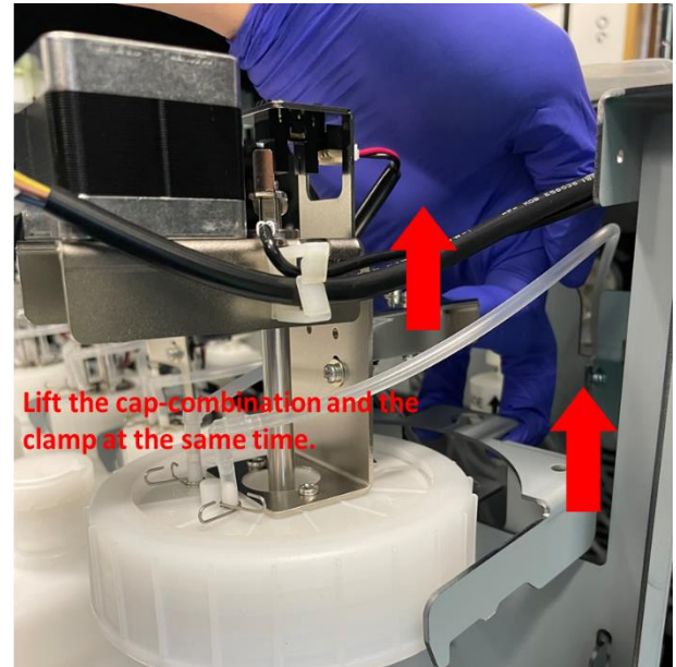
Figure 3. Lift the cap and clamp combination.
