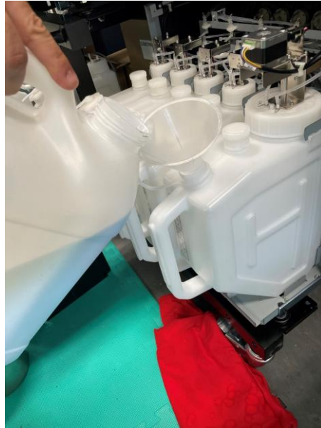
Figure 5. Adding ink to the main tank.
