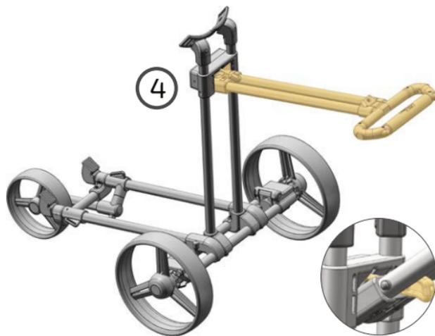
Bring handle in position and adjust if necessary.
