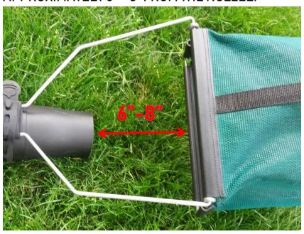
8. WHEN PROPERLY INSTALLED THE BLOWER'S AIRFLOW SHOULD BE DIRECTED IN FRONT OF THE BAG.
