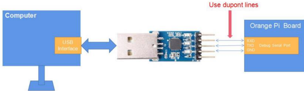
Schematic diagram of connecting USB to TTL module to computer and Orange Pi development board
