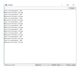
2. high speed ranging: Fast ranging, cost less time and low accuracy
