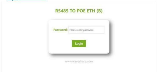
2. Enter a password in Password: There is no login password set by default in the factory, you can enter a password at will, and click the Login button to log in. After setting the password to log in, the settings at "Modify webpage login password" will take effect:
