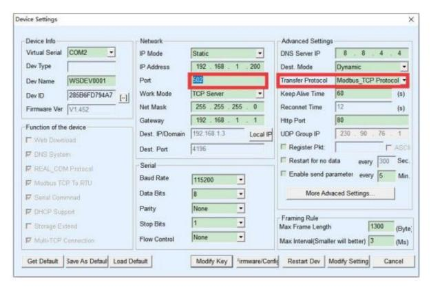
If the user's Modbus TCP software is used as a slave station (Slave), it is necessary to select the conversion protocol, then change the working mode to the client, the destination IP to the IP of the computer where the Modbus TCP software is located, and the destination port to 502, as shown in the figure below.
