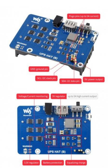
The 8.4V interface is the charging interface, which uses an 8.4V 2A power supply for charging. 5V OUT is a USB male port that can output 5V power. The 0FF/ON silkscreen is the power switch silkscreen.
