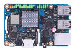
The performance of tinker board is much higher than most of the SBC boards, therefore the heat generation is also higher. But tinker board will comes with a passive heatsink to cool down the main SoC temperature.
