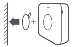
3. Hanging: Remove the back cover of the monitor, and lead the lanyard's loop through the hole and around the hook. Reinstall the back cover, then hang the monitor.
