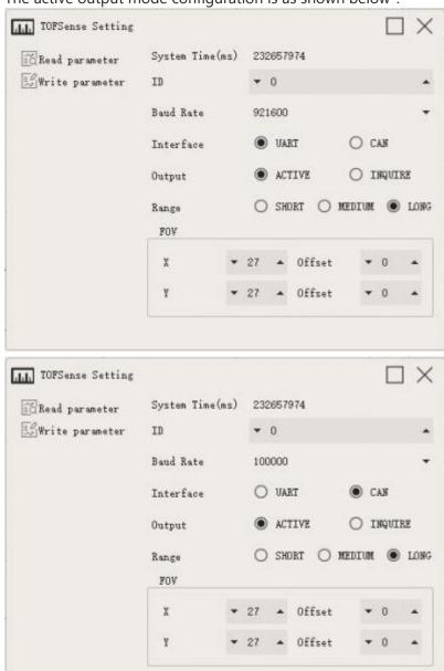
• The active output mode configuration is as shown below :
