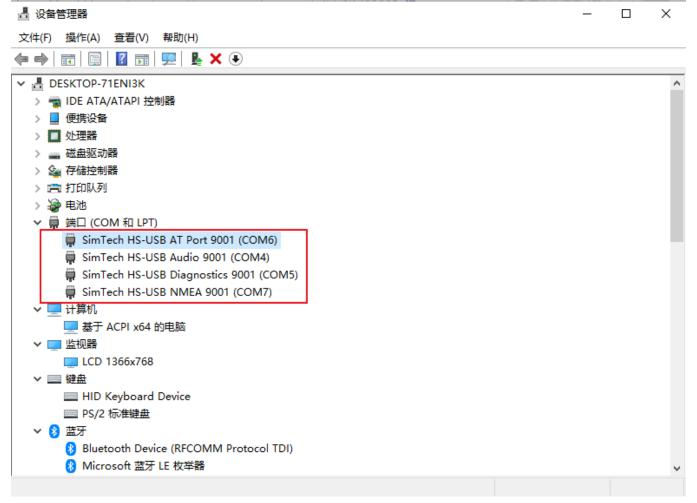
Four COM ports: AT is used for AT command controlling, and Audio is used for dail up. Diagnostics is used for debugging, and NMEA is used for GPS.
