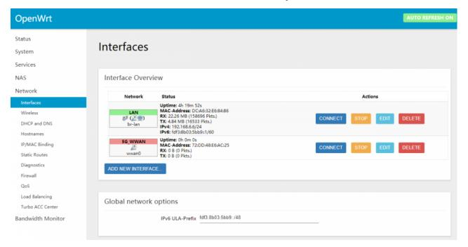
Then the other devices can be connected to the wireless "OpenWrt" or through the network cable to connect to OpenWrt's own network port for networking. In terms of the speed measurement, as the Raspberry Pi comes with a Gigabit Ethernet port, and there are few USB network cards above Gigabit, we use the "SpeedTest For Python" tool to test the speed with the command.
