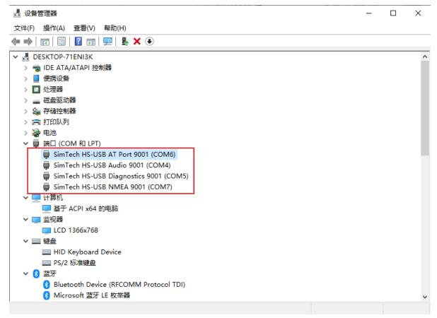
Four COM ports: AT is used for AT command controlling, Audio is used for dailing Diagnostics is used for debuggging, and NMEA is used for GPS.;
