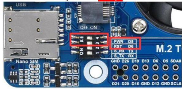
• **Power Control:**The following demonstrates the Shell script to control the PWR (D5 PIN) as an example:
