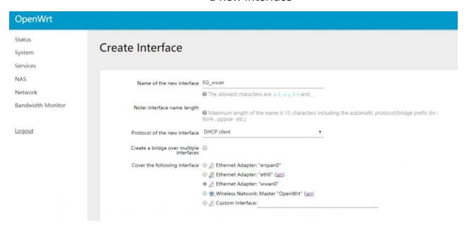
Enter the interface as shown in the picture below and confirm that the interface selection in "Physical Settings" is "wwan0".
